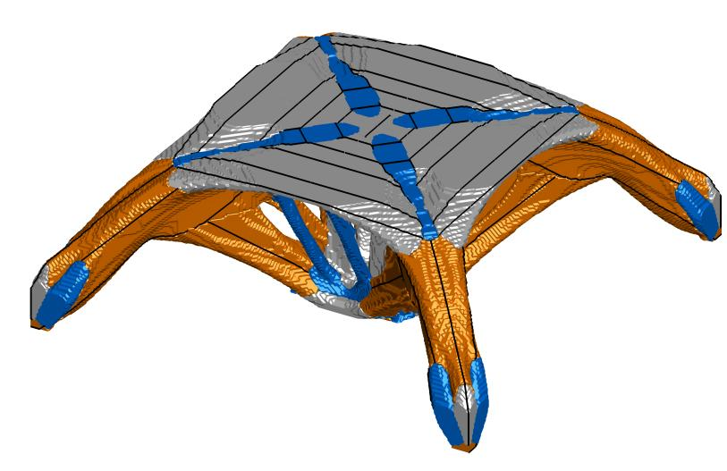
• Orthotropic design using AMR: 3.19 million elements with 5.91 million DVs
