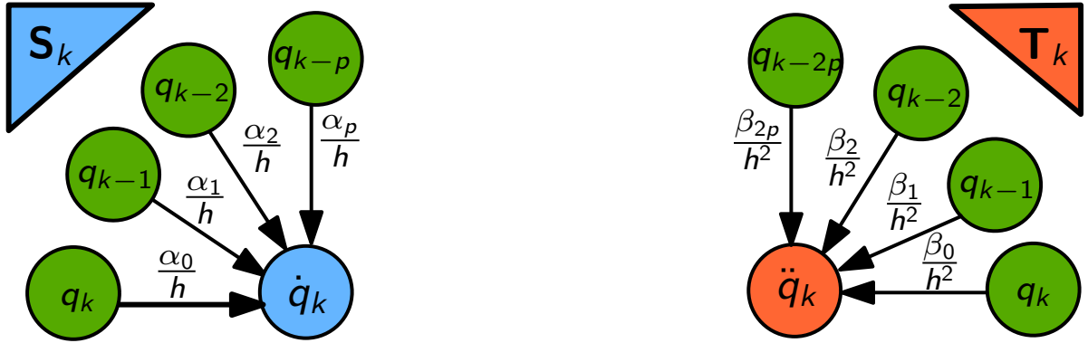
Figure 4.4: A weighted linear combination of the state variables with scaled BDF coefficients yielding the first (left) and second time derivatives of state variables (right). These relations are respectively labeled as the state approximation equations S_k and T_k .
