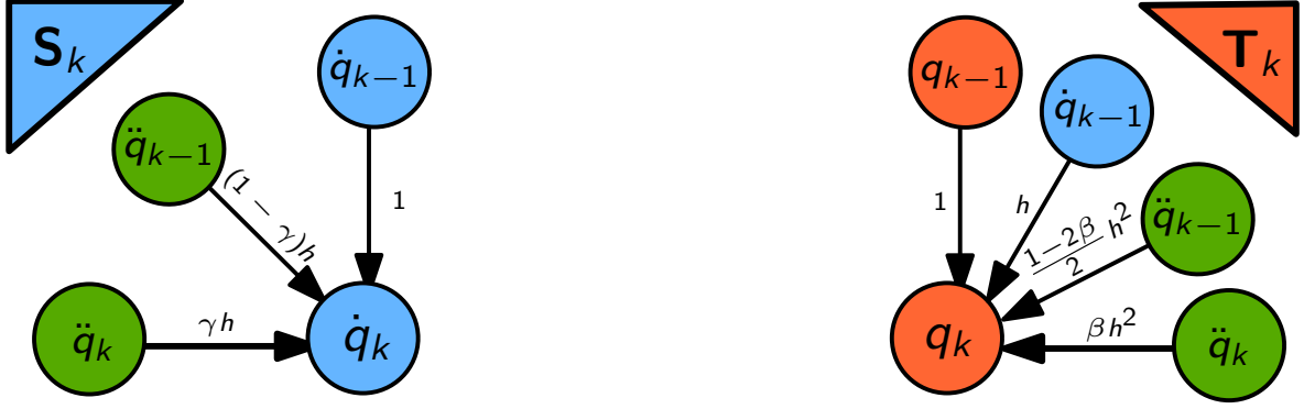
Figure 4.1: Weighted linear combination of states yielding the velocity (left) and position (right) states for Newmark method using state approximation hypothesis S_k and T_k .
