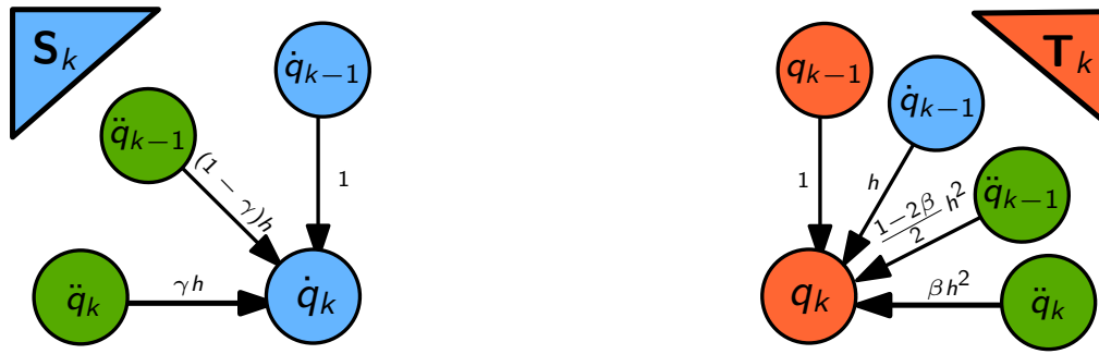
Figure 3: An illustration of weighted linear combination of states yielding the velocity (left) and position (right) states for Newmark method. These constitute the state approximation equations \mathbf{S}_k and \mathbf{T}_k .
