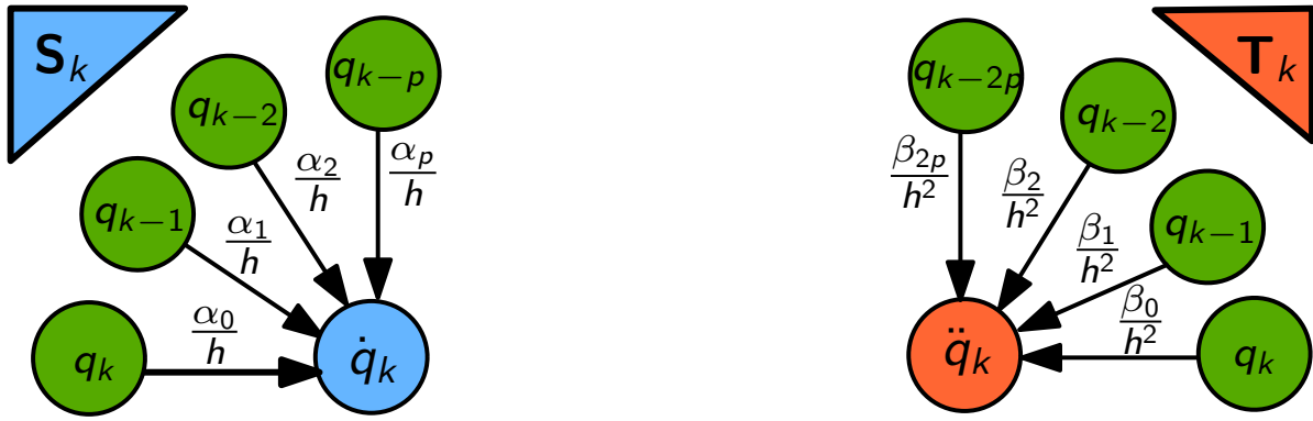
Figure 1: A weighted linear combination of the state variables with scaled BDF coefficients yielding the first (left) and second time derivatives of state variables (right), denoted as state approximation equations, \mathbf{S}_k and \mathbf{T}_k , respectively.
