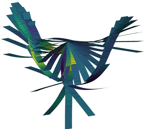
Figure 11: Time lapse of the flexible double-plate pendulum over the time history of the motion.
